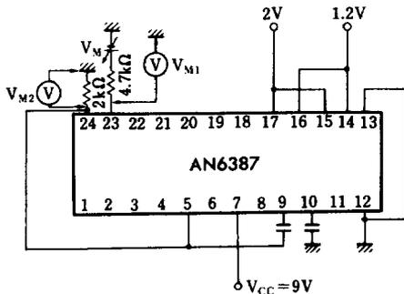
Set  $V_M$  at 2V. Continuously increase  $V_M$  until it is as shown in the figure below.
